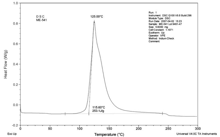
**Figure 6: DSC thermogram for cure profile of underfill**
