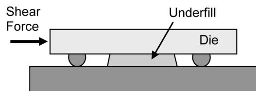
Figure 1: Diagram of die shear adhesion test assembly
