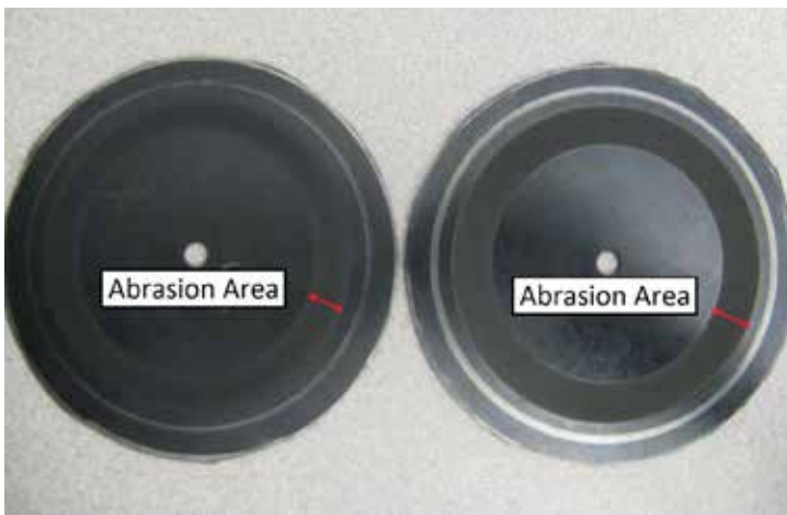
Figure 2: Examples of Abrasion Test Samples with indicated abrasion area
