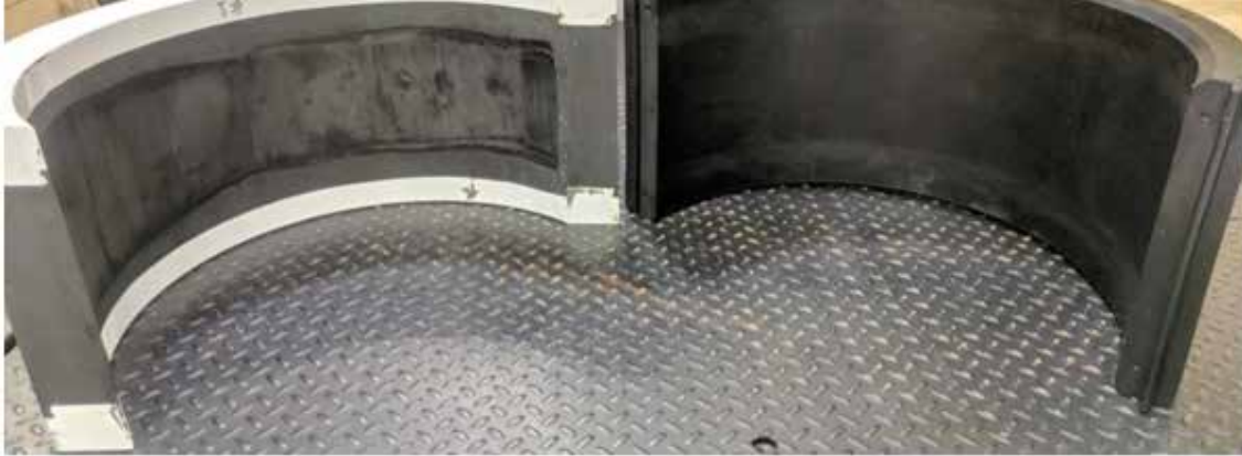
Figure 16: Standard Nitrile Packer elastomer crumbing due to abrasion
