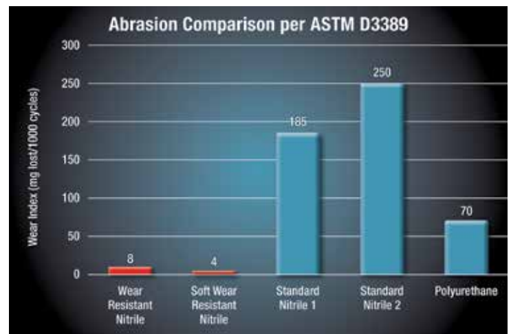
Figure 3: Material Specimen Rotary Platform Abrasion Testing Results
