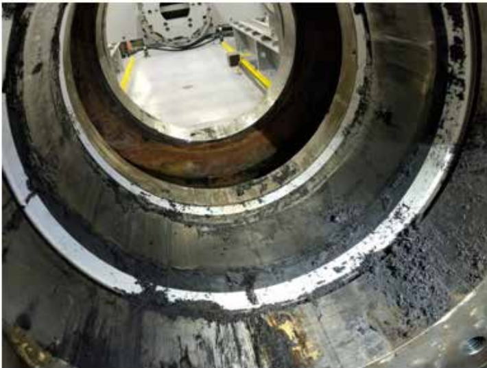
Figure 16: Standard Nitrile Packer elastomer crumbing due to abrasion
