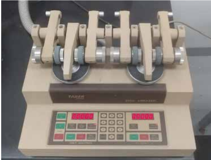
Figure 1: Rotary Platform Abrasion Tester used to perform comparative abrasion testing on two elastomer specimens at a time
