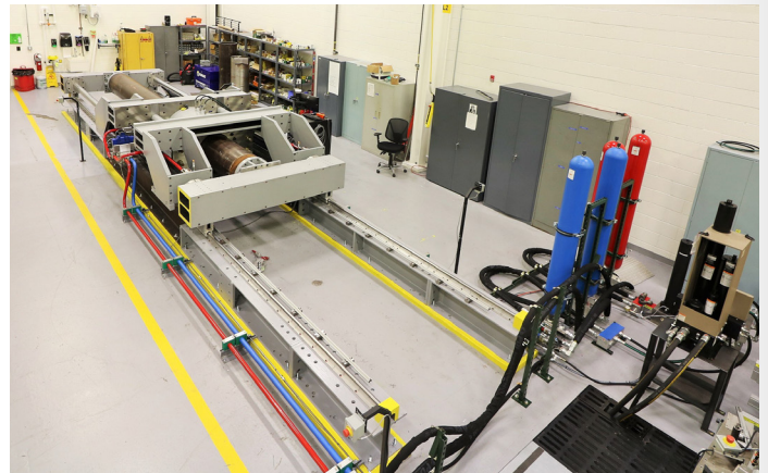
In-house test fixture for certifying TJ packers to API 16F and for durability testing
