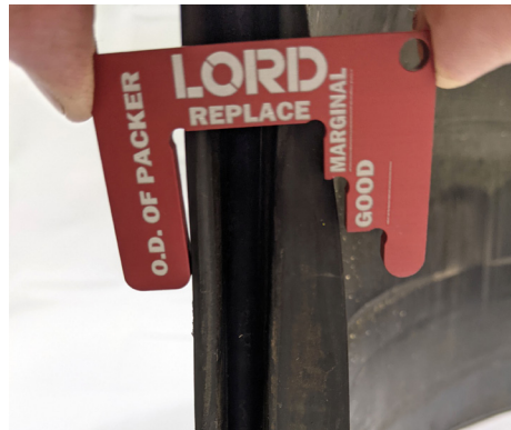
Figure 5. Wear Gauge Use - MARGINAL Elastomer Thickness
