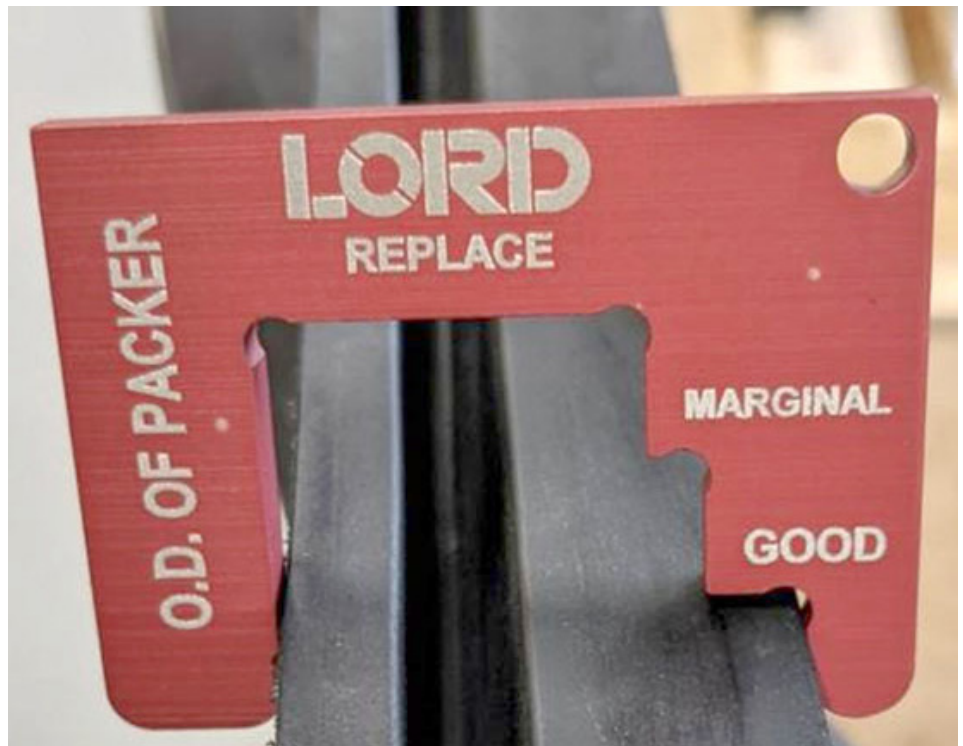
Figure 3. Packer Wear Gauge on New Packer
