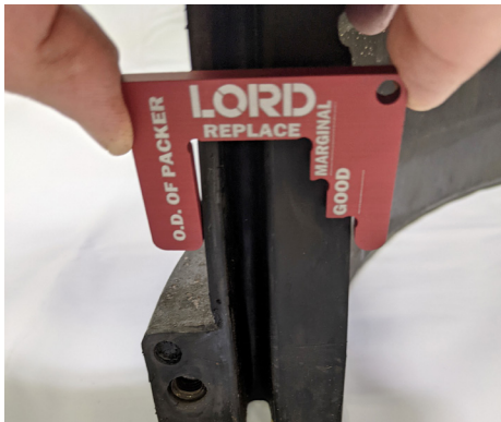
Figure 4. Wear Gauge Use - GOOD Elastomer Thickness
