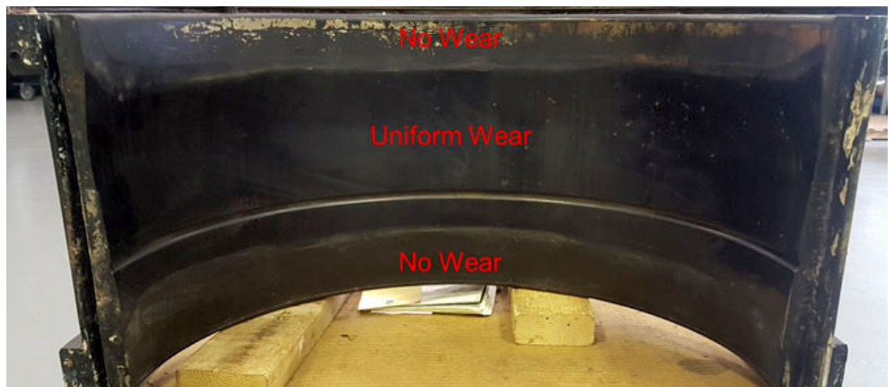
Figure 2. Packer Typical Wear Location
