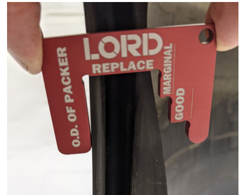
Figure 6. Wear Gauge Use - REPLACEMENT Elastomer Thickness
